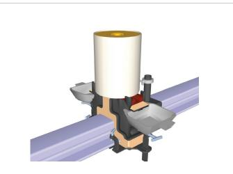
The arrangement for welding. The refractory sand mould is held in place around the rail with clamps. The disposable crucible is protected in a cardboard tube. Excess slag from the casting process flows into the slag pans.
